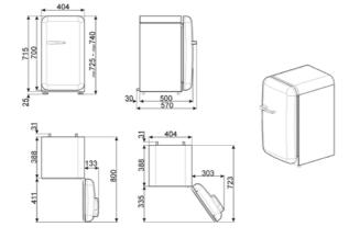
When positioning these appliances adjacent to a wall or kitchen unit a gap of 175mm must be left on the hinged side of the product to allow the door to open.
