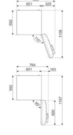
When positioning these appliances adjacent to a wall or kitchen unit a gap of 175mm must be left on the hinged side of the product to allow the door
