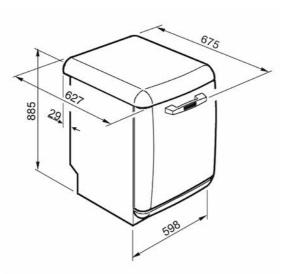
NB: This dishwasher will not fit under a standard worktop. Please check measurements carefully and choose the built-in version if there is insufficient height.
