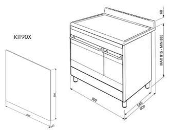
NB: Height with plinth installed is fixed at 900mm
