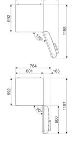
When positioning these appliances adjacent to a wall or kitchen unit a gap of 175mm must be left on the hinged side of the product to allow the door to open.
