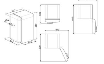
When positioning these appliances adjacent to a wall or kitchen unit a gap of 175mm must be left on the hinged side of the product to allow the door to open.
